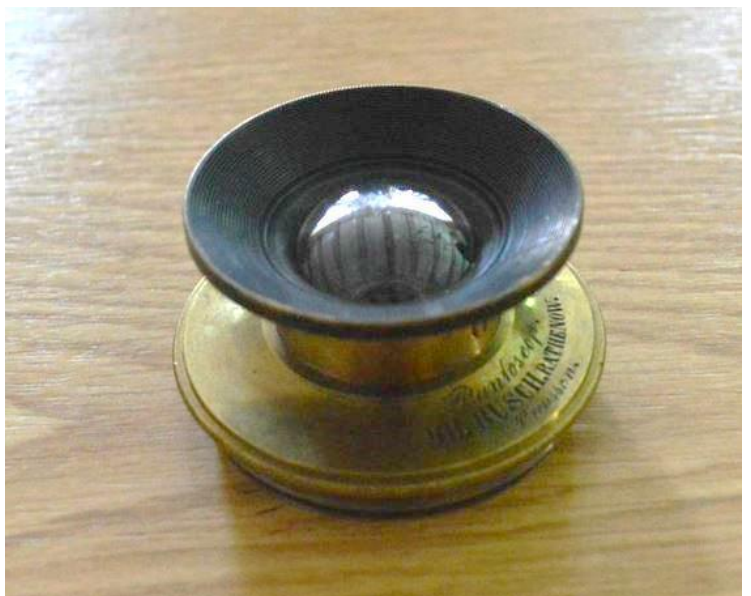
Figure 14, One of the very early lenses, used in Albrecht Meydenbauer's photogrammetric cameras
