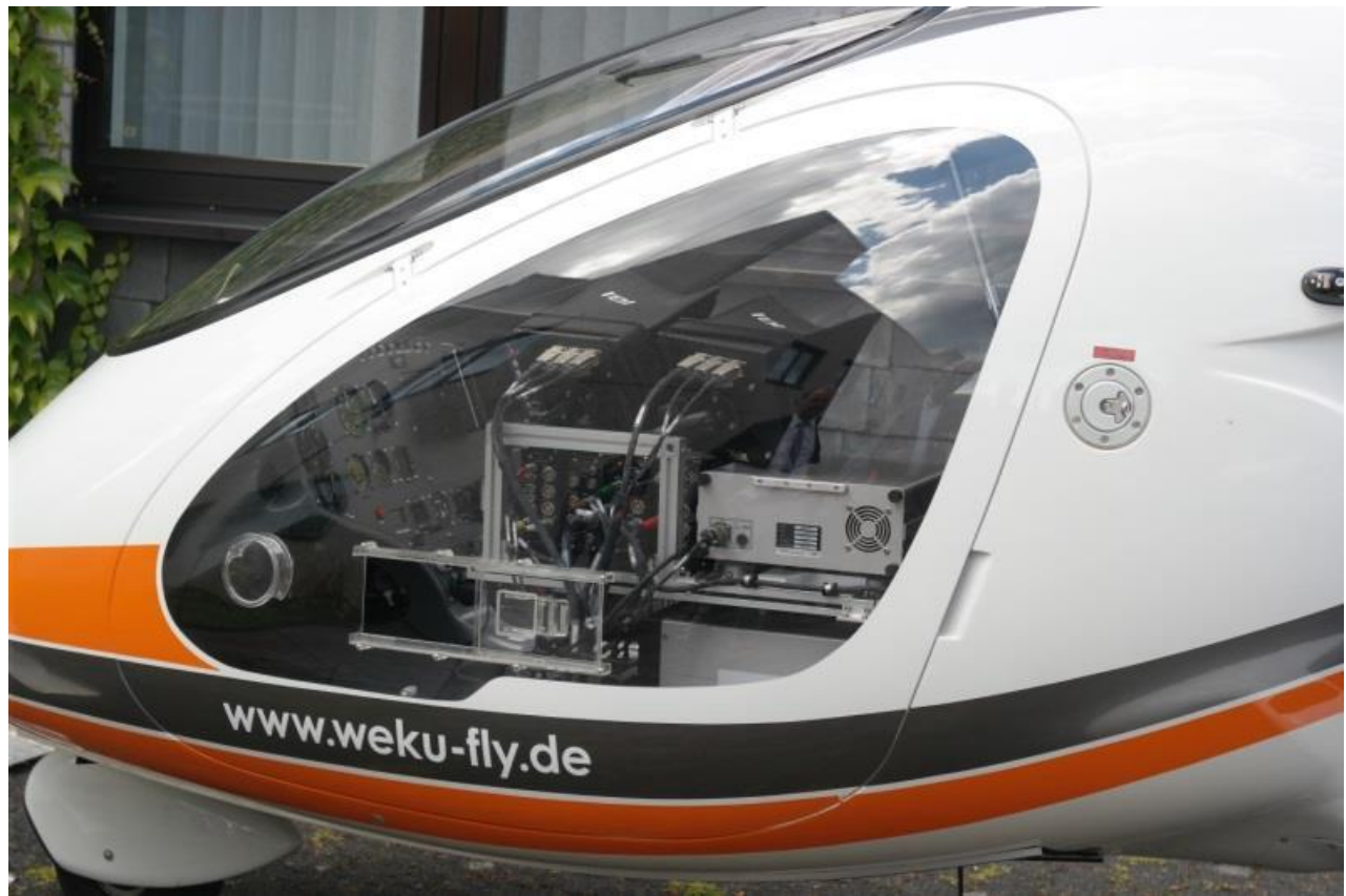
Figure 5, The Gyrocopter cockpit with IGI mobile mapping equipment.
