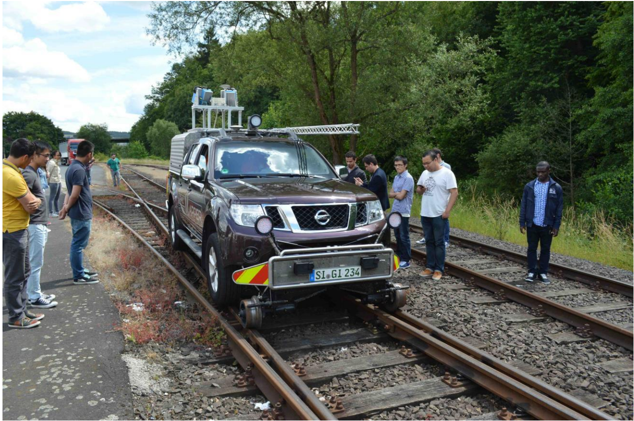
Figure 3, Railmapper after railing on the track
