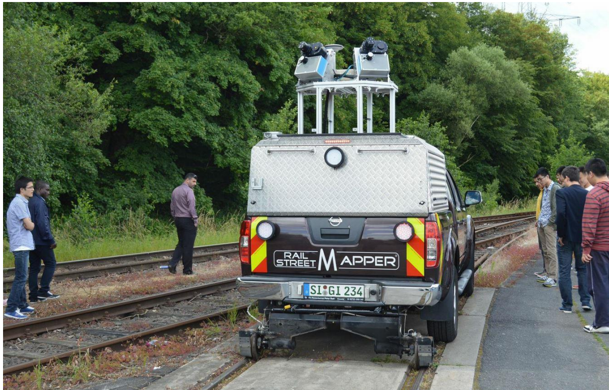
Figure 4, The Rail Mapper Measurements equipment on the roof of the two-way-vehicle
